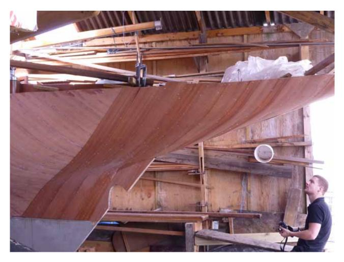
WBTA member Tim Loftus – www.timloftusboatbuilding.co.uk – uses wood-epoxy methods for both restorations and new builds. Above: Over the years, the carvel planking on this 1950 28' (8.5m) Alfred Mylne Glen class had been sanded away to half of its original thickness, so she was sheathed with epoxy-glued utile veneers. Below L & R: This 11'6" (3.5m) lain Oughtred Guillemot is a new build in epoxy-glued clinker plywood, a method also used by CNC-cut kit manufacturers. Photographs: Tim Loftus.
